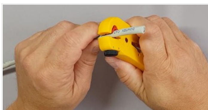
Strip 40mm of sheath from cable using stripper
