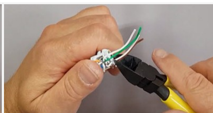
Using side cutters, cut the wires level with the wire forming cap
